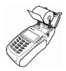
7. Close the paper roll cover by gently pressing directly on the cover until it clicks shut. Allow a small amount of paper to extend outside the cover (as shown below).
